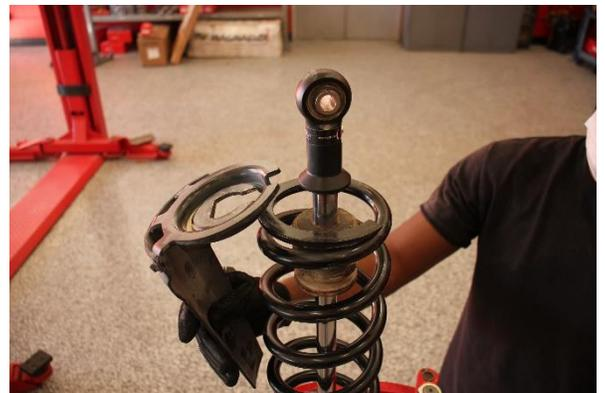
Step 6. Compress the coilover, then remove the spring retainer. **Note:** The bump stop will need to be pried down, out of the way of the spring retainer.
