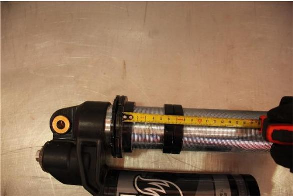
Step 9. Move the OE cross-over rings and set them at **80mm** measuring from the spring flange to the bottom of the crossover rings.
