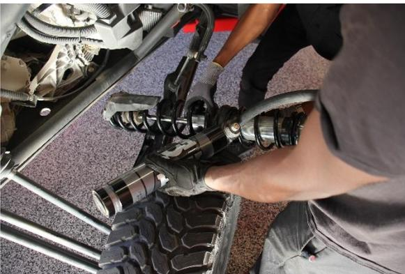
Step 5. Carefully guide the resi/resi hose through to hole in the bed, and remove coilover.
