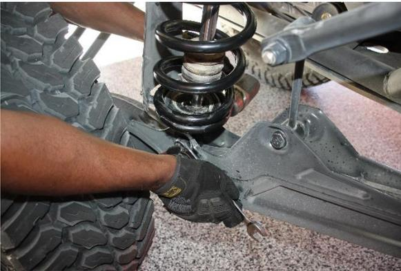
Step 3. Loosen and remove the hardware that secures the coilover to the control arm.
