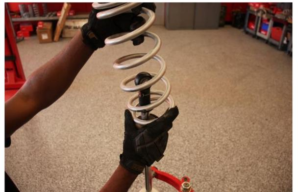
Step 12. Install the Eibach secondary spring.
