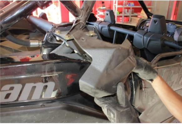
Step 1. Raise the rear of the vehicle and support it with the proper safety equipment. Remove the two T30 torx screws then remove the plastic cover. **Note:** Never work on or under a vehicle that is not supported by the proper safety equipment.
