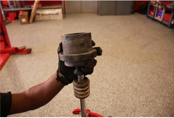
Step 13. Install the OE spring slider.
