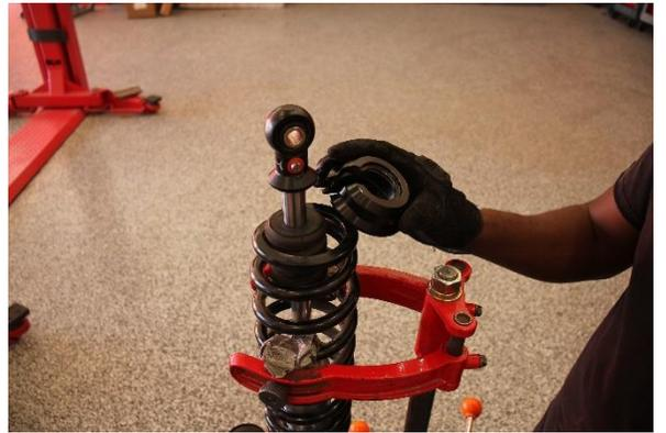
Step 4. Compress the coilover, then remove the spring retainer. **Note: The bump stop will need to be pried down, out of the way of the spring retainer.**
