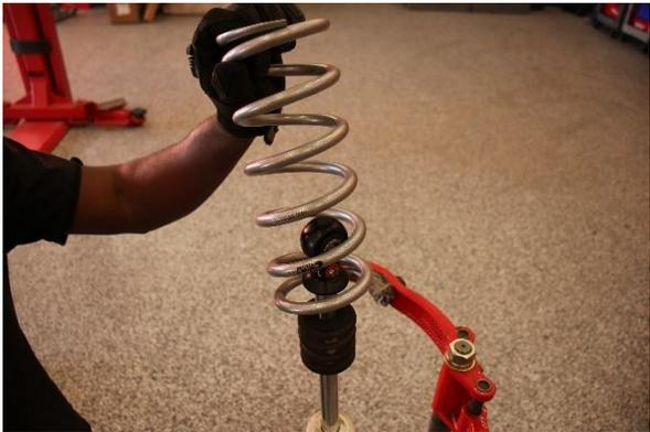
Step 10. Install the Eibach secondary spring.
