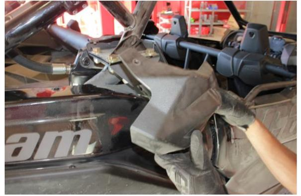
Step 20. Re-install the plastic cover fastened by 2 T30 screws.
