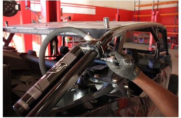
Step 2. Remove the 4 socket head cap screws on the resi mounting bracket, set resi in bed.
