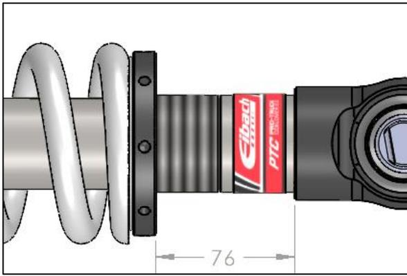
Not: Do **NOT** go above a spring perch height of 76mm or else damage to the shock and suspension will occur.
