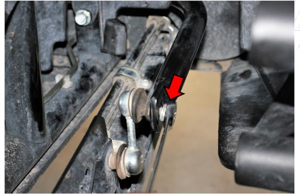
Loosen and disconnect the end link from the sway bar.
