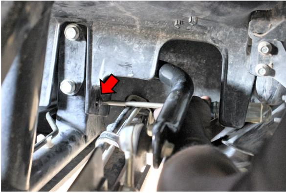
Begin by removing the screw holding the plastic to the frame near the bracket on both sides.
