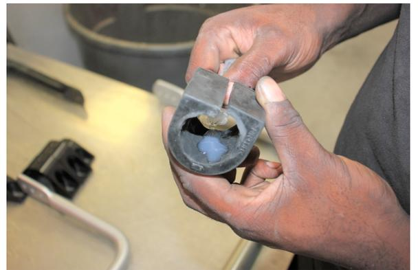
Lubricate the new bushings with the provided grease before installing on the Eibach sway bar.
