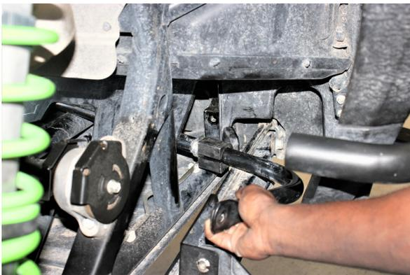
Once all the hardware is removed you can remove the OE sway bar.
