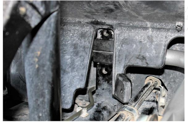
Make sure the new bushings are properly installed into the opening in the frame.
