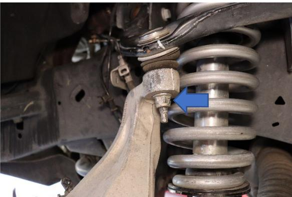
Step 4. Loosen the upper ball joint nut.
