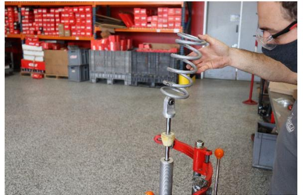
Step 10. Install the Eibach secondary spring (0800.300.0300S).
