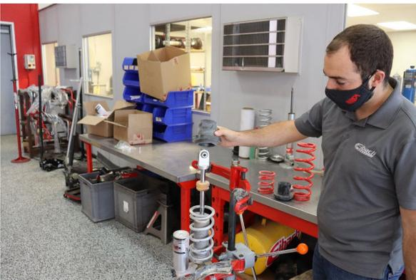
Step 11. Install the Eibach spring slider (8001498).
