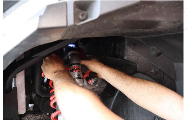
Step 2. Loosen and remove the hardware that secures the coilover to the upper mount.
