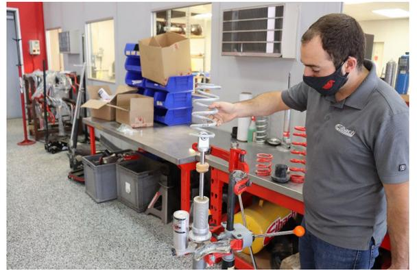
Step 10. Install the Eibach secondary spring (0800.300.0350S).
