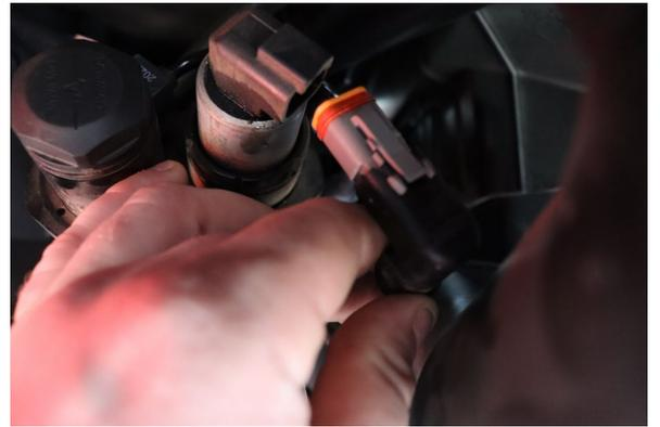
Disconnect the both electrical connectors for the Live Valve.
