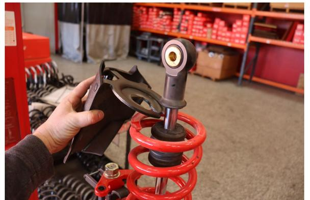
Compress the springs and remove the OE spring seat.
