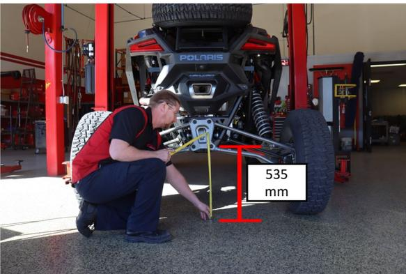
With the vehicle back on the ground, drive the car to settle the suspension and measure the height from the ground to the lower radius rod bolt. This should measure approximately 535mm with a stock 32" tire and no extra weight added. Changing tire size or adding weight will affect this measurement.
