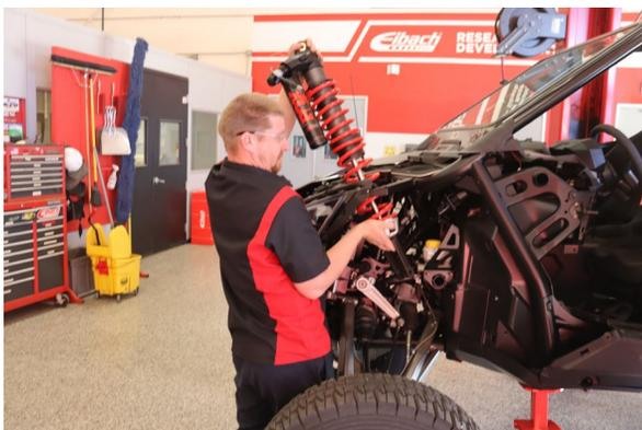
Pull the shock up through the top. It may help to twist the shock body first to align the reservoir with the opening.
