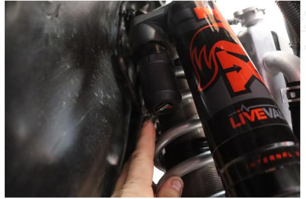
Plug in the electrical connector at the top of the coilover.
