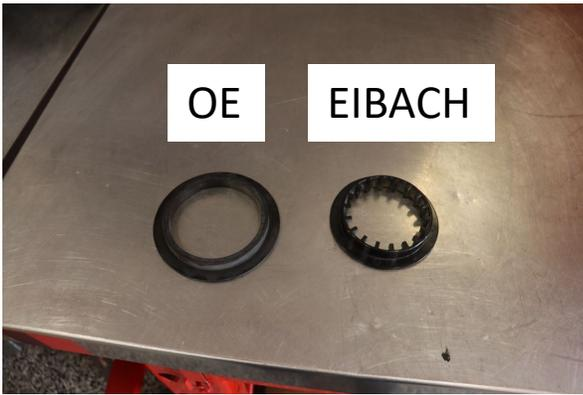
Remove the OE Spring adapter and replace with the provided one. Then reinstall the crossover ring and slider sleeve with the clips.
