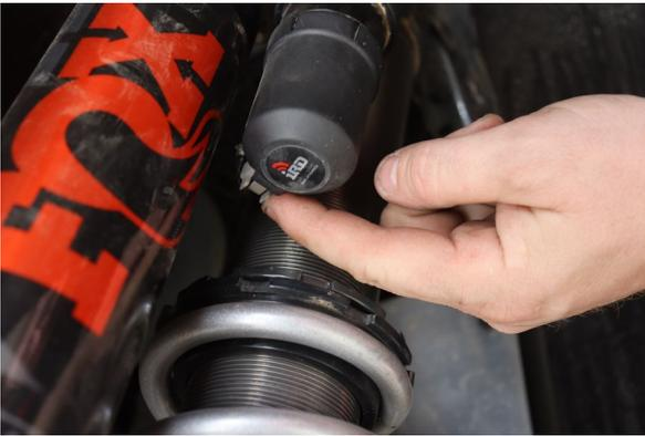
Remove electrical connector from the top of the coilover.
