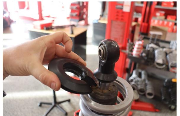
Step 5. Compress the coilover, then remove the OE spring retainer. **Note: The bump stop will need to be pried down, out of the way of the spring retainer.**
