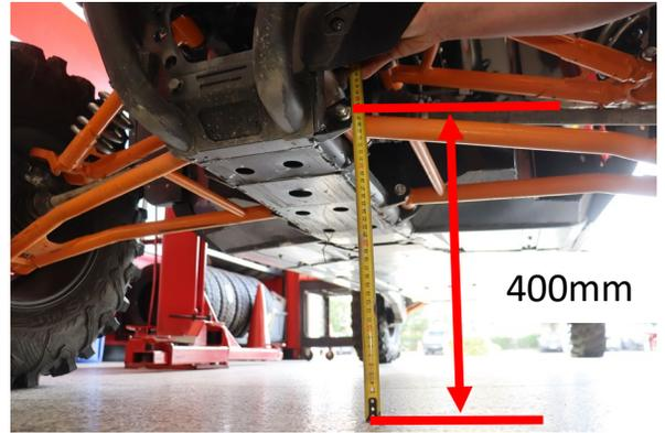
Lower vehicle back to ground and measure from the ground to the center of the lower control arm bolt. The recommended preload measurement will get the vehicle close to the recommended ride height with weight added to the vehicle, but each vehicle may vary some. We recommend setting the ride height at **400mm** measuring from a flat surface to the center of the lower control arm bolt.. Front shock length is approximately **735mm** eye to eye at ride height
