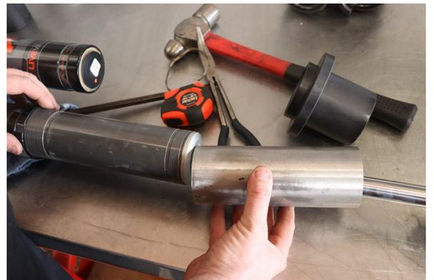
Remove the slider sleeve and crossover rings.
