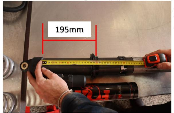
Set the preload collar to 195mm measuring from the base of the reservoir housing to the spring perch.
