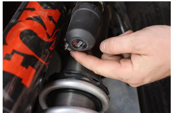
Reinstall the connectors at the top of the shock for the Live Valve and complete on the opposite side.
