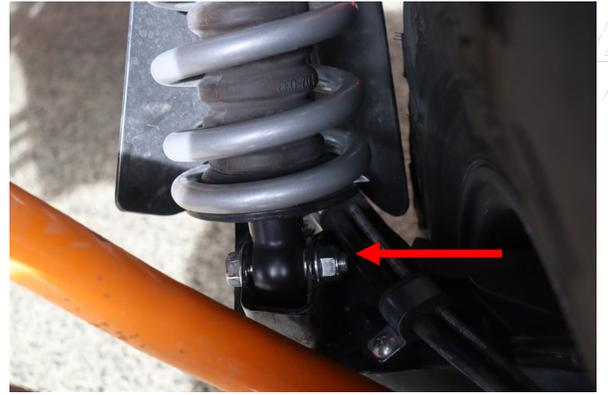
Loosen and remove the hardware that secures the coilover to the control arm. **Note: Never work on or under a vehicle that is not supported by the proper safety equipment.**
