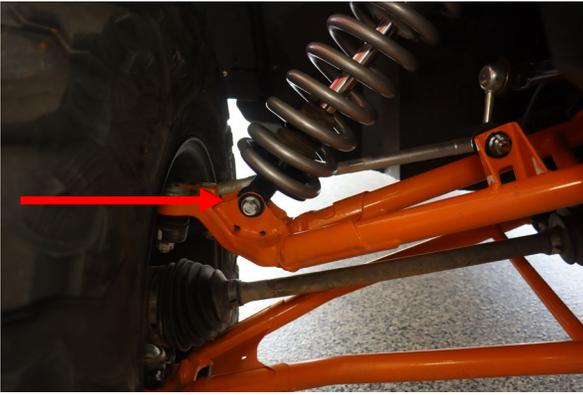
Secure the coilover to the control arm with the OE hardware.
