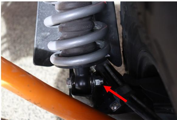
Install the bolt connecting the shock to the lower control arm.
