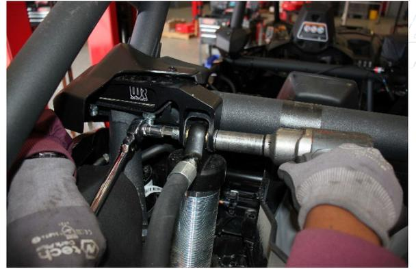
Step 2. Loosen hardware on the top mount, but do not remove the bolt.
