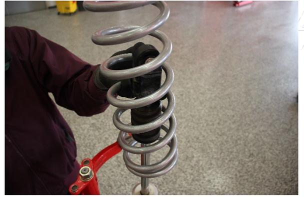
Step 14. Install the Eibach secondary spring.
