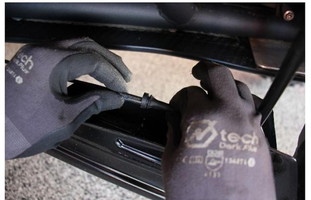
Step 4. Remove electrical wire from arm hold down to give enough slack to remove connector.
