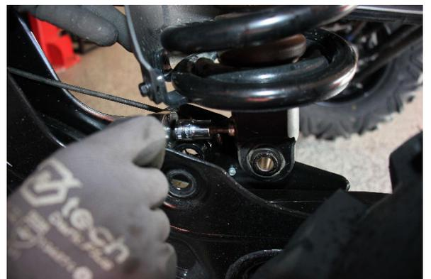
Step 6. Swing bottom of the shock out of the mounting clevis on lower control arm, remove two allen screws and pull electrical connector out of the bottom of the shock. **Note: Be careful not to get dust/dirt inside of the electrical connector. Do not stretch wire as damage can occur.**
