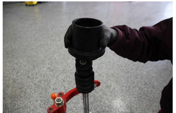
Step 12. Install the OE spring slider.
