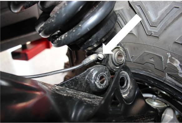
Step 3. Swing bottom of the shock out of the mounting clevis on lower control arm, remove two allen screws and pull electrical connector out of the bottom of the shock. **Note: Be careful not to get dust/dirt inside of the electrical connector.**
