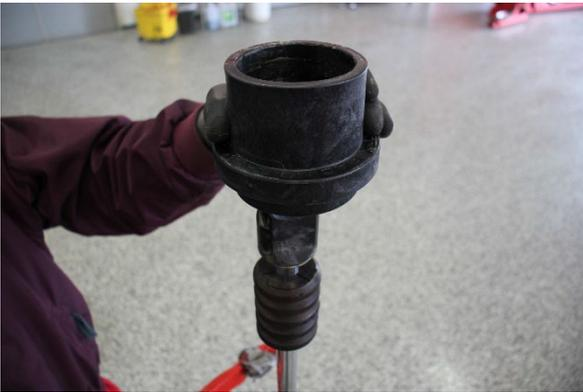
Step 15. Install the OE spring slider.
