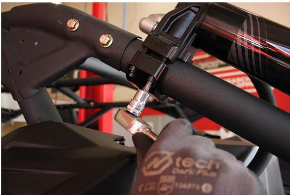
Step 3. Remove the 4 socket head cap screws fastening the resi to the cage. Place the resi in the bed.
