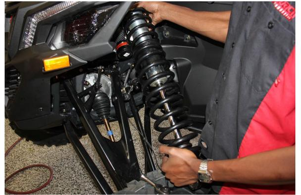
Step 4. Remove bolt from upper mount and remove coilover.
