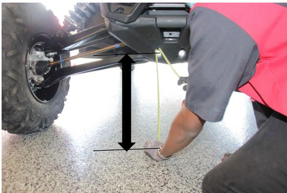
Step 19. Measure from the ground to the center of the lower control arm bolt. The recommended preload measurement in **Step 9** will get the vehicle close to the recommended ride height but each vehicle may vary some. We recommend setting the ride height at **475mm** measuring from the ground to the center of the lower control arm bolt. Shock eye to eye length should measure about 715mm **Note: If you have larger than stock wheels and tires, the ride height will be increased.**
