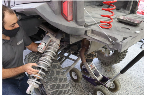
Step 14. Reinstall the coil over.
