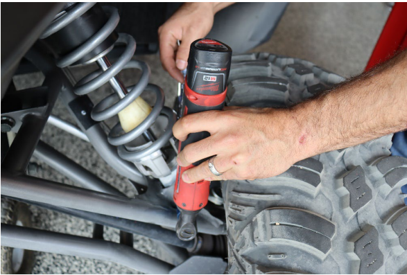
Step 15. Secure the coilover to the control arm with the OE hardware.
