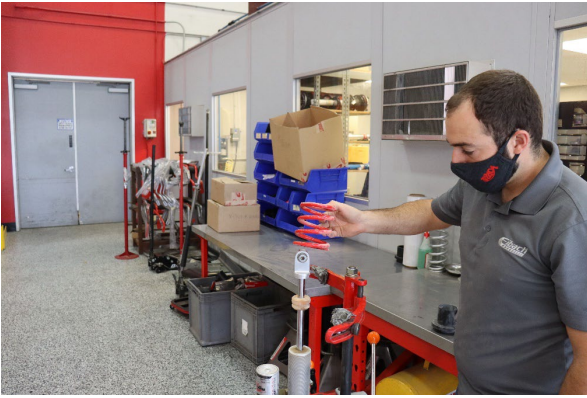
Step 7. Remove OE secondary spring.
