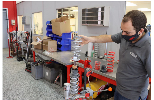
Step 12. Install the Eibach main spring (1000.300.0350S).
