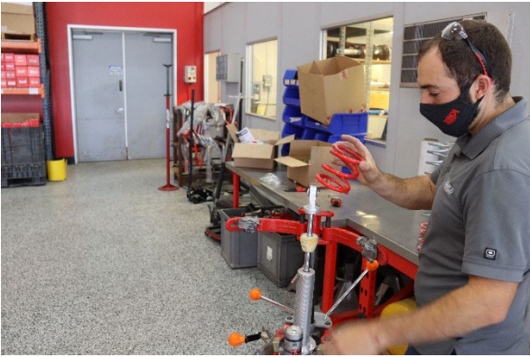
Step 7. Remove OE secondary spring.
