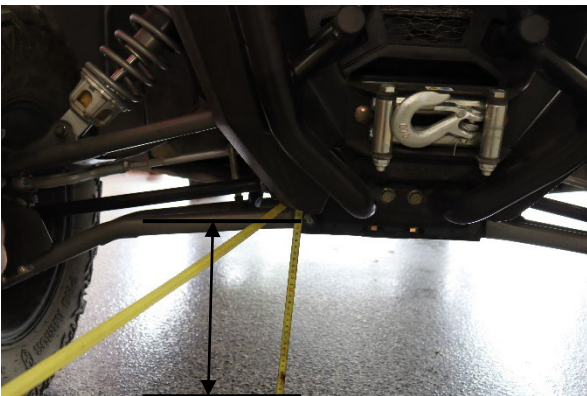
Step 16. Measure from the ground to the center of the lower control arm bolt. The recommended preload measurement in Step 8 will get the vehicle close to the recommended ride height but each vehicle may vary some. We recommend setting the ride height at 415mm measuring from the ground to the center of the lower control arm bolt. Note: If you have larger than stock wheels and tires, the ride height will be increased. Due to the sensitivity of weight on these vehicles, preload may need to be adjusted to get to recommended ride height.
