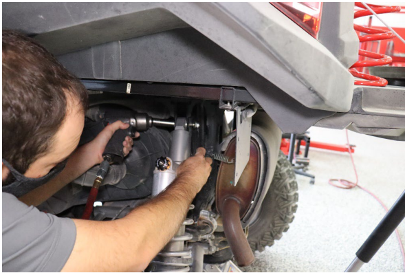
Step 15. Secure the coilover to the upper mount with the OE hardware.
