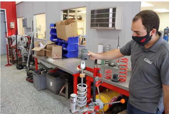
Step 11. Install the Eibach spring slider (8001498).
