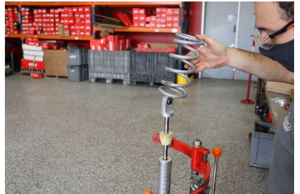
Step 10. Install the Eibach secondary spring (0800.300.0300S).
