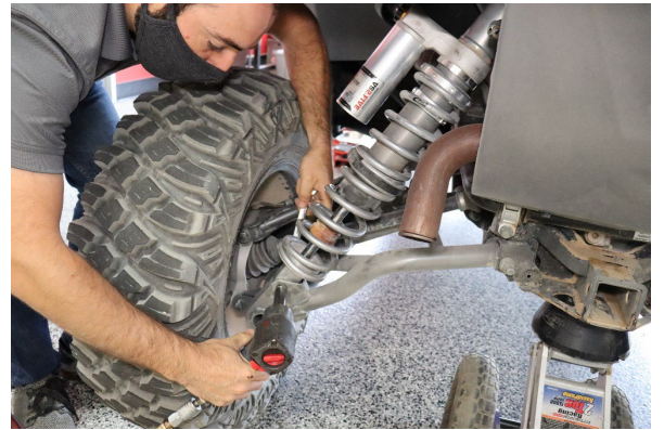
Step 16. Secure the coilover to the control arm with the OE hardware.
