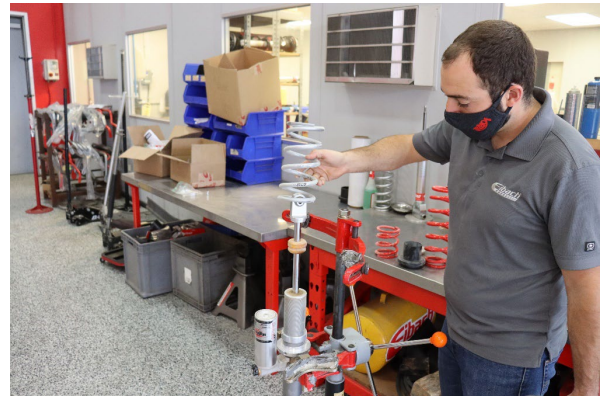
Step 10. Install the Eibach secondary spring (0800.300.0350S).
