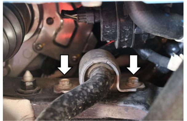
4. Remove the two bolts that secure the OE bar with a 15mm socket.
