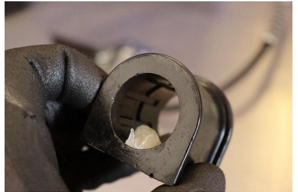
10. Apply the lubricant to the bushing
