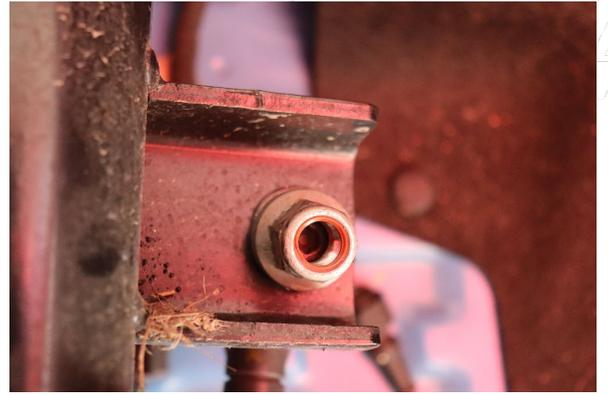
2. Remove the nut that secures the end link with an 18mm socket.
