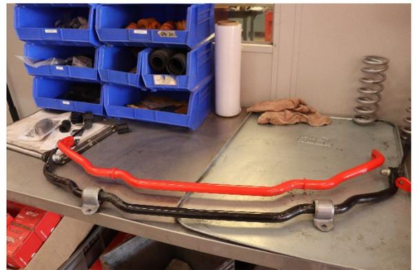
6. Confirm the orientation of the Anti Roll bar with the OE bar.
