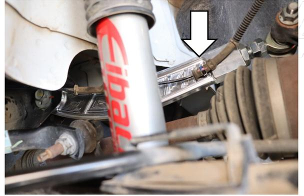
Step 3. Reinstall the wheel speed sensor wiring to the camber arm.
