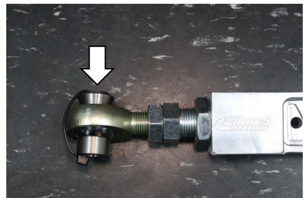
Before installing ensure that the tapered heim spacer is facing the knuckle of the vehicle.
