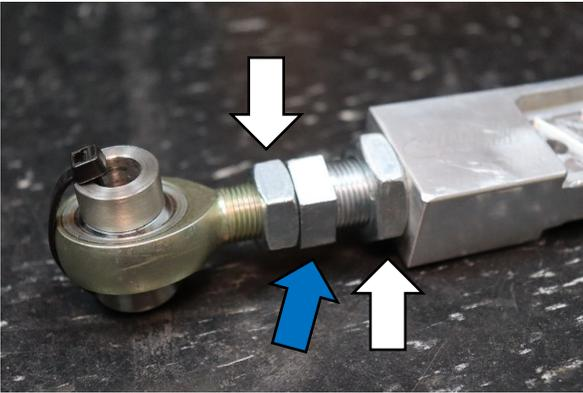
When making adjustments make sure the threads are equal by rotating from the center adjuster only. (Blue) DO NOT extend arm past 380mm eye to eye
