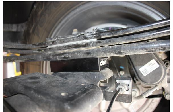
Raise the axle so the locating pin on the bottom of the leaf springs is located in the hole on the top of the lift block
