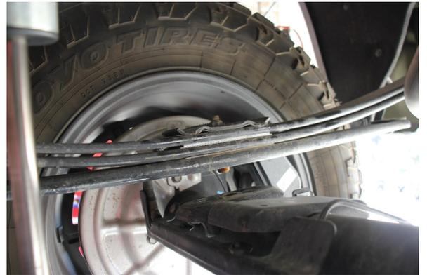
Lower the axle enough to insert the new lift block
