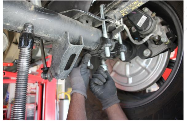
Install the OE axle carrier and the provided washers and nuts and hand tighten so each end is evenly tightened. Do not tighten completely at this point.
