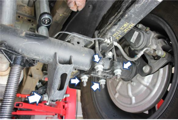
With the vehicle raised and properly supported loosen and remove the hardware securing the lower shock mount and the 4 nuts and U-bolts securing the axle to the leaf spring
