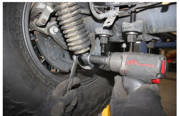
Reinstall the lower shock bolt.
