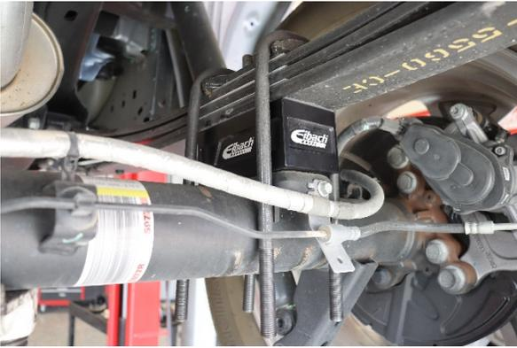
Raise the axle back up so the pins are fully seated on the top and bottom of the block and then reinstall the provided u-bolts.
