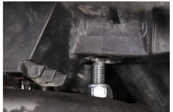
**Step 12:** Tighten the three flange nuts from the strut assembly top hat to the shock tower (43 ft-lbs).
