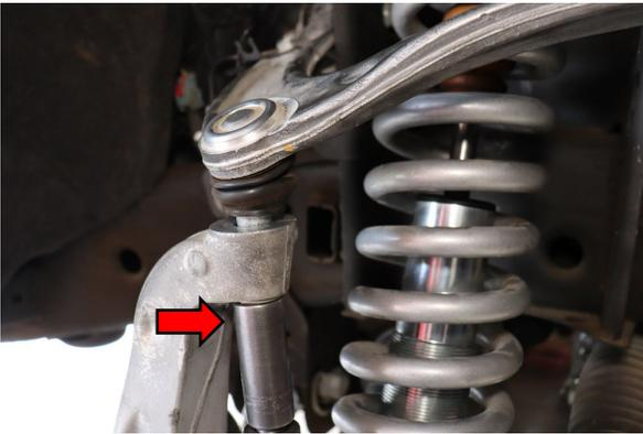
**Step 15:** Lower the Upper Control Arm into the steering knuckle. **Note: The Upper Control Arm contains bushing preload and will need to be held in place using a pry bar.** Once in the proper position secure the arm with the 18mm nut and tighten to 89 lb-ft then a 45-60 degree turn.
