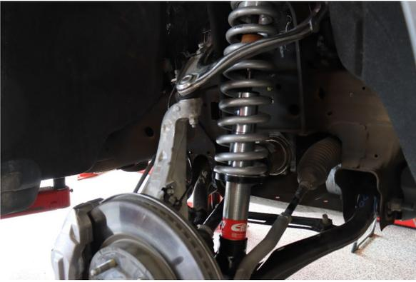
**Step 19:** This concludes the installation of the Pro Truck Coilover 2.0. Ensure that all your hardware is properly installed before reinstalling the wheels.
