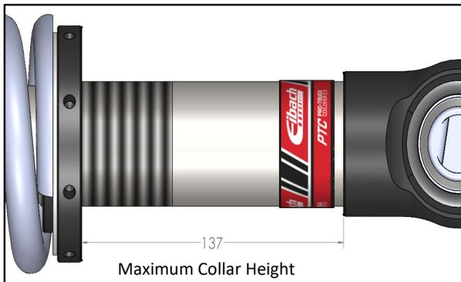
**Note:** Do NOT go above a spring collar height of 137mm from bottom of collar to base, as shown or else damage to the shock and suspension will occur.
