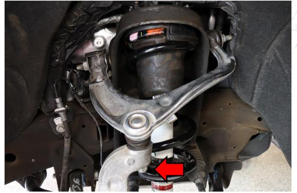
**Step 8:** Loosen, but do not remove the 18mm nut to separate the upper control arm from the steering knuckle. **The upper control arm is preloaded and may swing upwards upon nut removal, use a pry bar to keep force applied to the UCA, remove the nut and slowly let the UCA swing up.**
