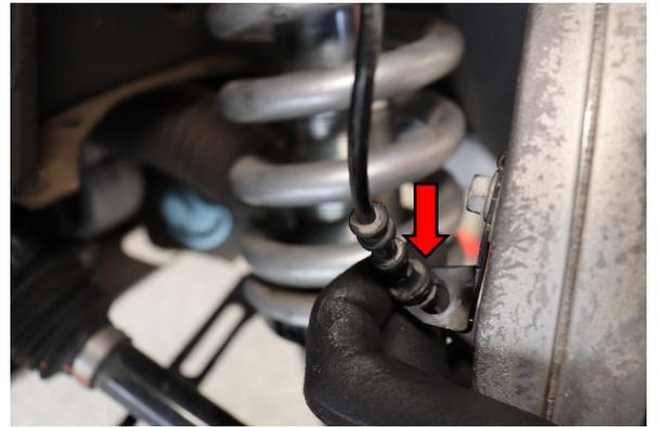
**Step 16:** Reinstall the wheel speed sensor grommet into the bracket
