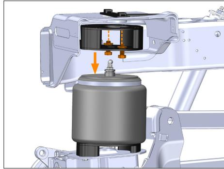
Carefully separate the air spring from the upper bracket and compress the air spring by pushing down on it.
