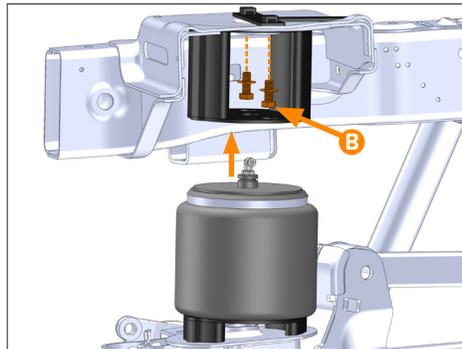
**B** Re-install the two 1/2" bolts with some threadlocker and torque to **75 FT. LB.**
