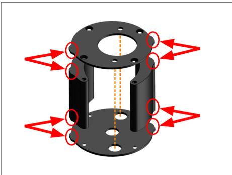
The two plates of the upper bracket should be oriented so the 1/2" holes on the upper plate line up with the clearance holes on the lower plate.
