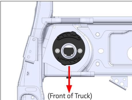
Ensure the upper bracket is in the orientation shown before installing the bolts.
