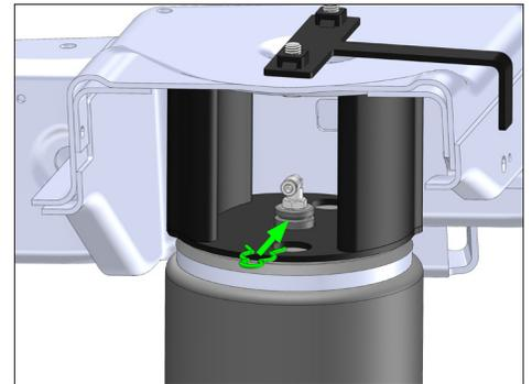
Re-install the hairpin clip in the groove of the air spring.
