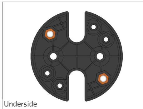
Press a 3/8" hex spacer in the two hex holes, on top of the nuts, as shown. This will secure the nuts in the hex holes.
