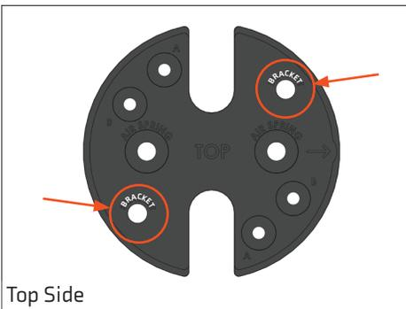
For the final spacer in your stack, place a 3/8"-16 nut in the two hex holes on the underside of the lift spacer that correspond to the holes marked "BRACKET" on top of the lift spacer.
