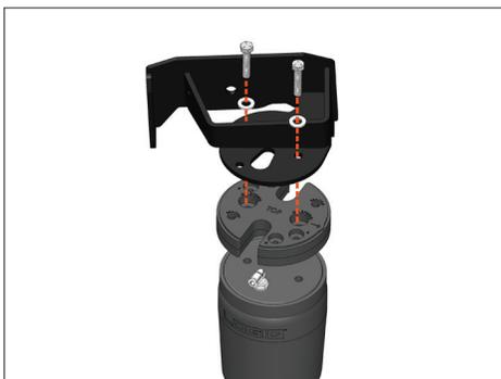
Bolt one lift spacer between the air spring and upper bracket using the "AIR SPRING" holes and supplied 1.75" long 3/8" bolts with flat washers. Apply some threadlocker to each bolt.
