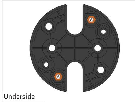
Place a 1/4"-20 nut in the two hex holes on the underside of the lift spacer that correspond to the holes marked "A" on top of the lift spacer.
