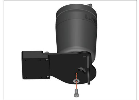
Unless installing a 1" lift, remove the one 3/8" bolt holding the lower bracket to the air spring and remove from vehicle.
