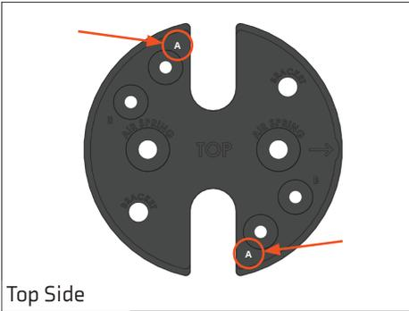
For 2-6 inch lifts, the lift spacers need to be prepped with hardware before assembling to the air spring.
