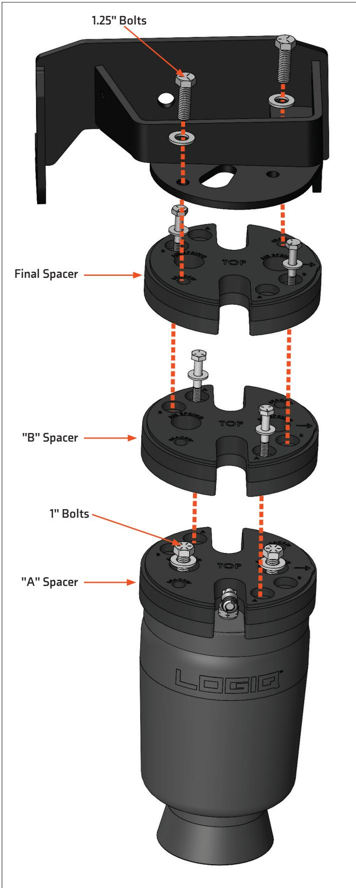
**⚠ TORQUE EACH SET OF HARDWARE BEFORE INSTALLING THE NEXT SPACER/BACKET.**
