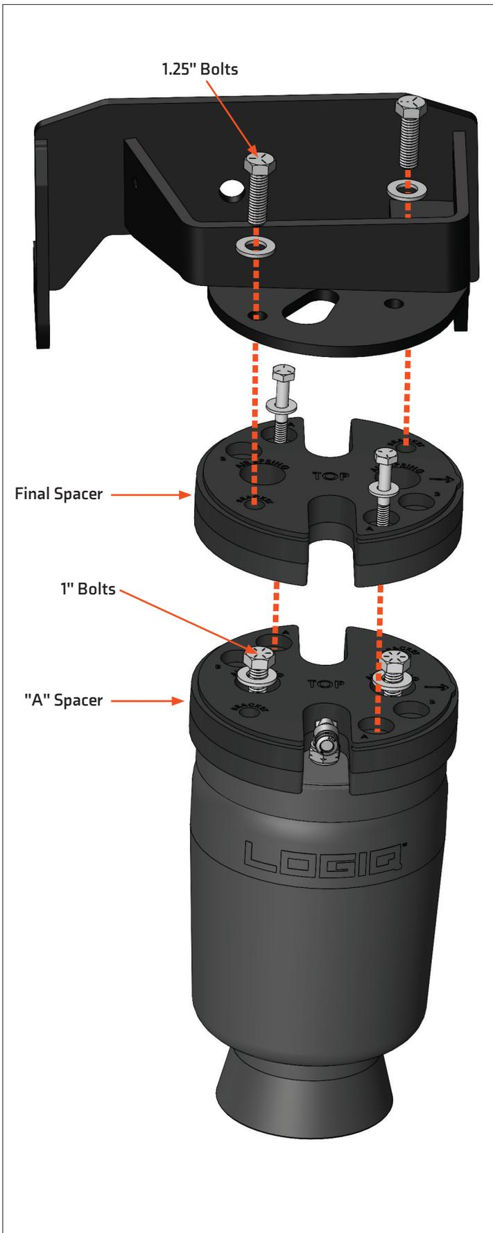
**⚠ TORQUE EACH SET OF HARDWARE BEFORE INSTALLING THE NEXT SPACER/BRACKET.**
