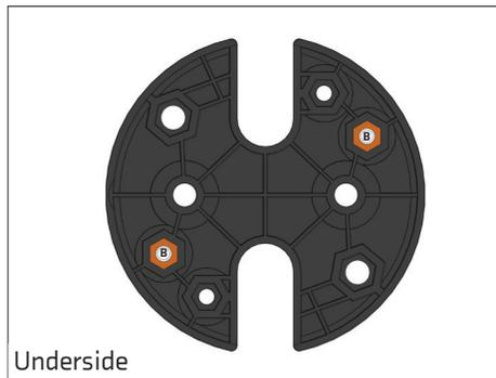
Place a 1/4"-20 nut in the two hex holes on the underside of the lift spacer that correspond to the holes marked "B" on top of the lift spacer.
