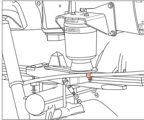
**NOTE:** Ensure that the E-brake cable has adequate clearance and is not making contact with any components.
