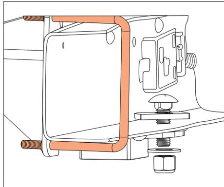
Install the 3/8" U-bolt with washers & nuts so that it is clamping around the frame.
