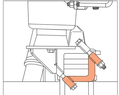
Secure the lower bracket to the leaf spring with the supplied 3/8" hardware and clamps. Make sure the bracket cut-outs are aligned with the U-bolt saddle, and the leaf spring bottom clamp is oriented correctly. Snug the hardware.
