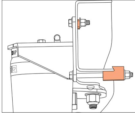
Install the upper 3/8" bolt with washers, nut and frame spacer. Ensure it is sitting flush against the frame. Install the lower 3/8" bolt with washers, nut and frame clamp. Ensure the clamp is sitting against the frame.
