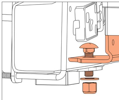
If using with an aftermarket 5<sup>th</sup> wheel bracket, install the carriage bolt WITHOUT the carriage bolt washer and instead through both the 5<sup>th</sup> wheel bracket and the upper bracket.
