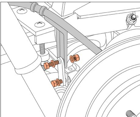
Once all fasteners are installed, use provided E-brake relocation bracket and install on driver side with provided M8 hardware. Torque to **8 FT. LB.**
