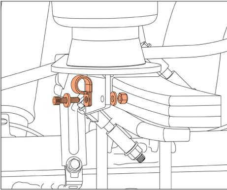
On the passenger side, bend and remove the factory E-brake bracket from the cable and fasten to the lower air spring bracket using the provided 5/8" Adel clamp and 1/4" hardware. Torque to **7 FT. LB.**
