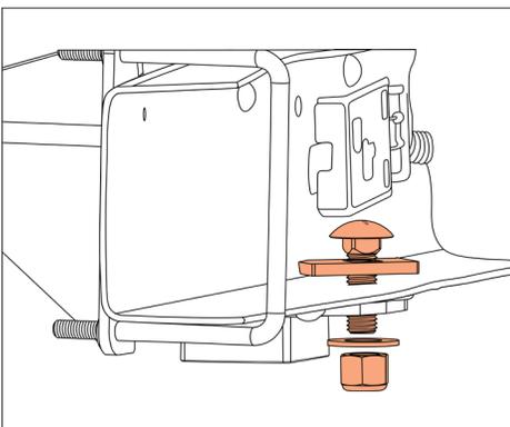
Install the supplied 5/8" carriage bolt and carriage bolt washer through the hole in the frame and the upper bracket.
