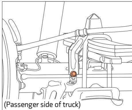
Un-bolt the emergency brake cable brackets on both sides of the truck.
