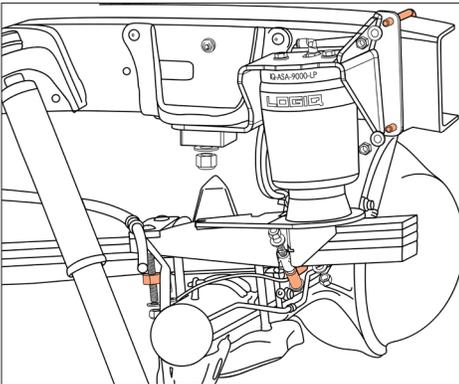
Driver assembly will be fastened with the U-bolt and lower bracket clamps in the orientation shown.
