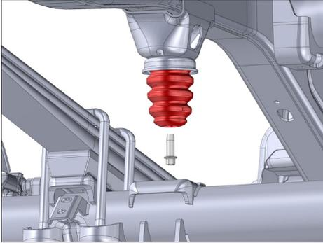
Un-bolt the factory bump stop using a 10MM socket and extension.
