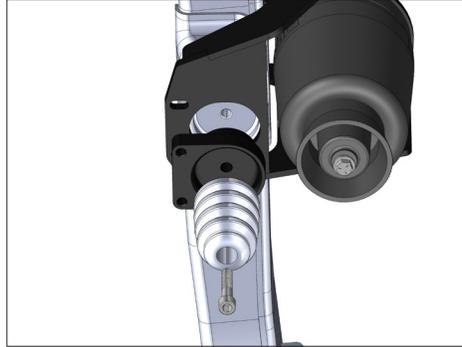
Slip the bump stop into the cup on the provided bump stop spacer.
