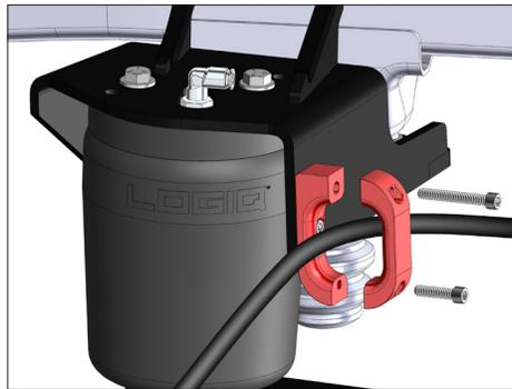
Route the E-brake cable through the middle of the base bracket. Secure the cap piece of the bracket to the base with the other two 1/4" screws (longer of the two goes in the top hole) to capture the E-brake cable.
