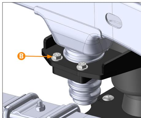
**B** Torque the 3/8" bump stop spacer hardware to **44 FT. LB.** using a 9/16" crowsfoot.
