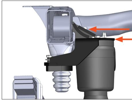
Push the upper bracket against the frame and snug the two 3/8" bolts.
