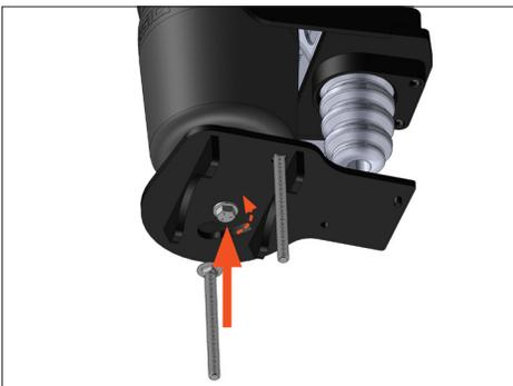
Install the 3/8" carriage bolts into the holes on the lower bracket, then apply downward force to extend the air springs and bring the lower bracket near the axle.
