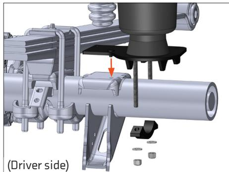
Attach the axle clamp. Make sure the pin on the lower bracket is aligned with the hole in the bump stop pad and the carriage bolts are parallel with the lower bracket leg before snugging.
