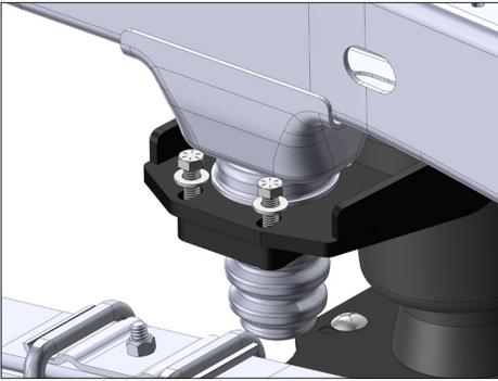
Go back to the upper bracket and install the provided 3/8" Grade 8 hardware into the bump stop spacer as shown.
