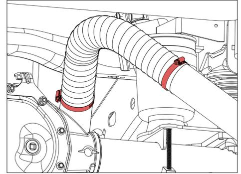
Once the **whole roll** has been wrapped onto the exhaust, attach the provided hose clamps to each end of the wrap as shown.
