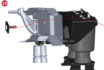
Check tire clearance to air spring (more than 1")
