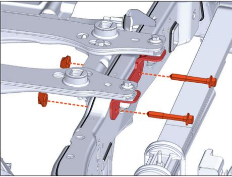
First remove the 5th wheel frame mounting hardware.
