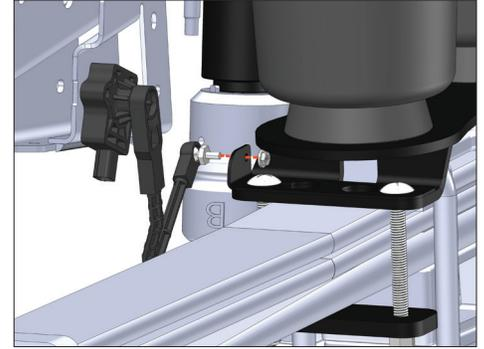
Attach the height sensor linkage arm to the relocation bracket using the factory nut.
