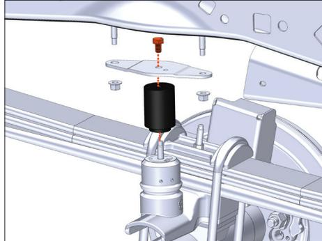
Reinstall factory bumpstop with provided aluminum spacer and M10 bolt.
