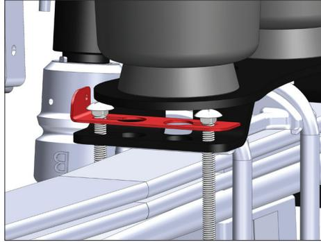
When attaching the lower air spring bracket, install the height sensor relocation bracket between the carriage bolts and the lower bracket leg.
