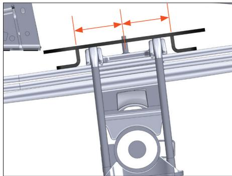
Make sure that the lower bracket is centered over the U-bolt saddle.
