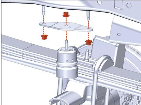
Unbolt factory bumpstop using a 15MM socket.
