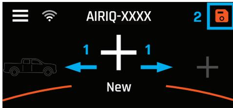
Save up to 8 preset pressure settings to fit different vehicle loading or use cases. To save a new preset, simply manually inflate/deflate to the desired pressures, then slide the carousel to the desired position and press **>SAVE**. Name the preset and associate it with an icon from the list.
