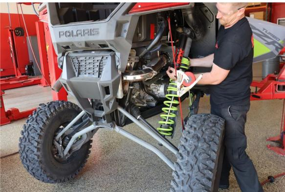
Remove the rear shock assembly.
