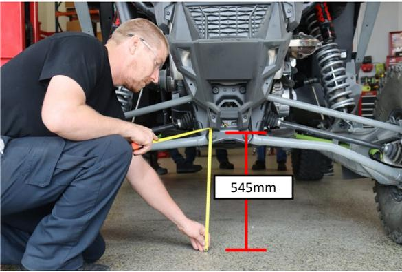
The rear ride height should be about 545mm from the ground to the lower radius rod bolt. Ride heights are measured without any extra weight on the vehicle. Extra weight will result in a lowered ride height.
