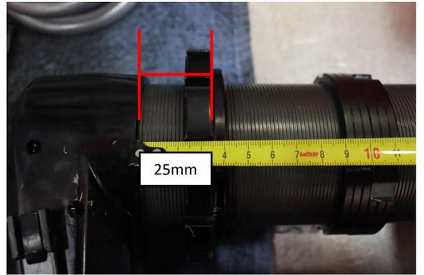
Set the preload collar to 25mm from the bottom of the reservoir to the spring seat on the preload collar
