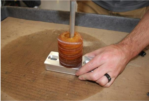
3. Use the M10 x 1.5 x 30mm bolts to secure the provided Eibach bump stop to the Eibach bump stop mount as shown.
