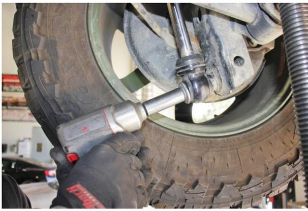
7. Loosen and remove lower shock bolt.
