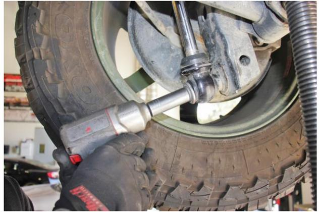
16. Secure the shock mount to the axle using the OE hardware as shown.
