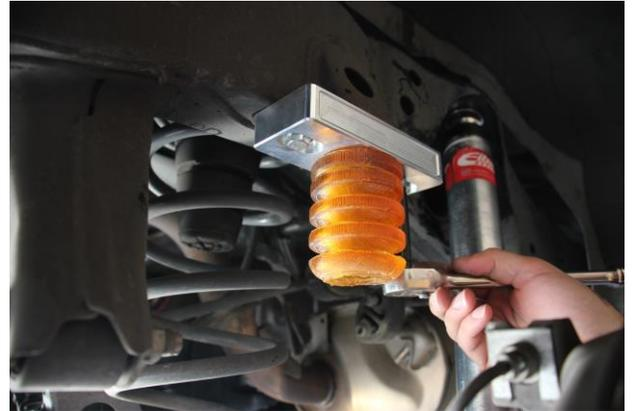
4. Install the new bump stop assembly using the M8 x 1.25 x 60mm bolts and M8 flat washers as shown.
