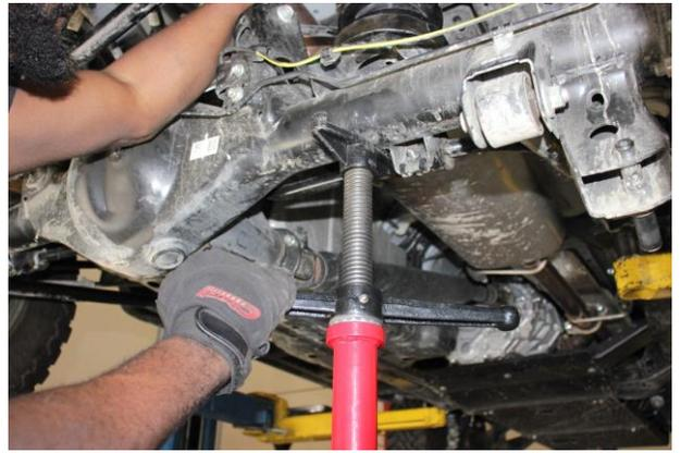
14. Compress the spring enough to install the lower mount of the shock to the axle.
