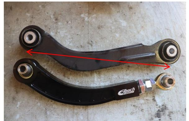
Set the Eibach Camber Arm to the same length as the OE camber arm before installation. Lock the jam nuts in positions once at the correct length. (This will be adjusted again later on an alignment rack.)
