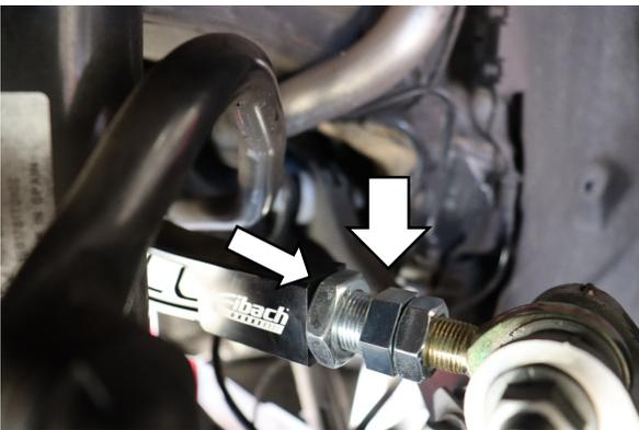
When adjusting the rear camber loosen the 24mm and 29mm jam nuts to adjust the rear camber of the vehicle. When the desired result is achieved lock the jam nuts back in place.
