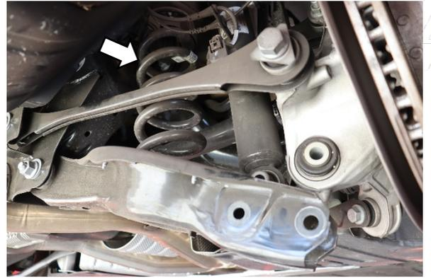
Reinstall the spring and support the lower control arm with a jack
