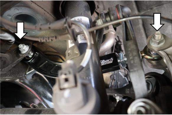
Install Eibach Camber Arm with the OE 18mm bolts.
