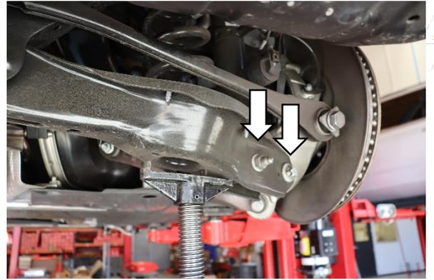
Support the lower control arm with a jack, then, remove the E20 bolt and 18mm nut. With the bolts completely removed lower the lower control arm.
