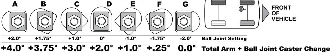
**Note: With SPC logo facing the tire (Position D) this arm will give +2° additional caster. Using the star plate, caster change can be adjusted from +0.0° to +4.0°.**
