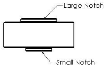
4. Install the shock with the selected notch placing the shock mount in between the pin bushings.
