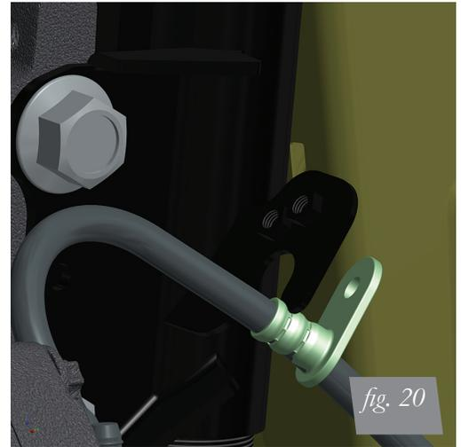
9. Attach the brake line and ABS sensor wire to the strut (Fig. 20). Torque the brake line bracket bolt to 9Nm (80 lbs.-in.).
