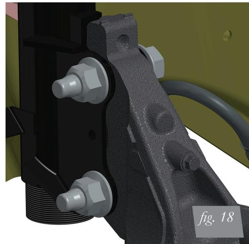
7. Lift the hub assembly and attach the assembly to the new strut. Torque the lower mount bolts to 80Nm + 180° (59 lb.-ft. + 180°).
