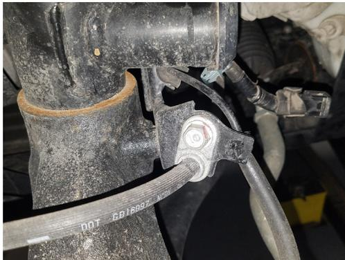
9. Remove the protective caps and install the provided Air Lift Performance end link onto the stabilizer bar and strut body tab. Torque the nuts to 64Nm (47 lb.-ft.).
