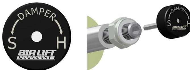
2. Turn the adjuster clockwise (H) and the damping settings are hardened, reducing oscillations and body motion. Turn the adjuster counterclockwise (S) and the damping is softened.
