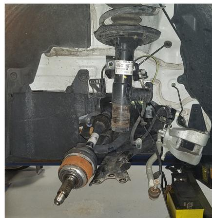
11. Remove the strut upper mount nuts and remove the strut from the vehicle.
