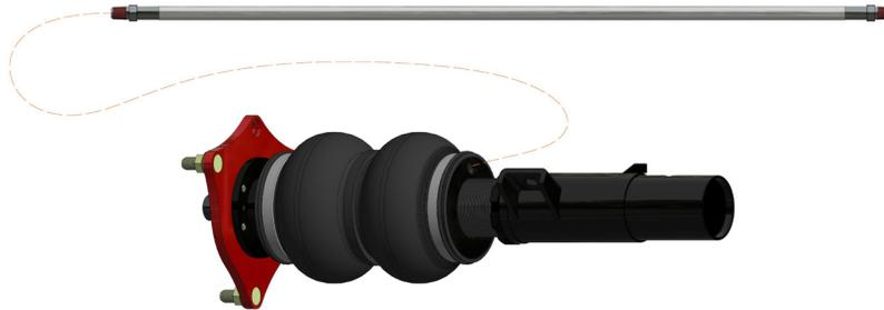
2. Insert the Air Lift Performance strut upper mount into the chassis and install the upper mount nuts. Ensure left-hand and right-hand struts are installed in the correct side. Torque the nuts to 75Nm (55 lb.-ft.).
