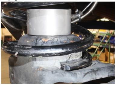
13. Use a Jack under the axle to compress the spring. If this is part of a Carli system, move on to the next instruction; otherwise, reinstall all components removed to install the springs.
