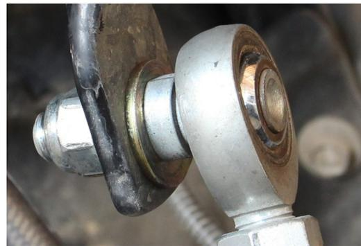
10. From the outside - in, The lower will be arranged: Sway Bar Link, 1/2" Gold Spacer, Axle Mount, Washer, Nyloc. **Torque to 75lb.ft.**
