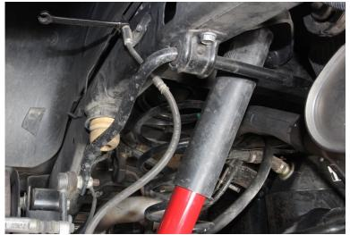
2. 15mm - Remove banjo bolt at caliper and remove the factory brake line.
