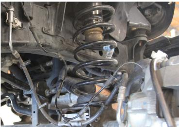
3. 12mm line wrench - Brake the hardline fitting at the frame.
