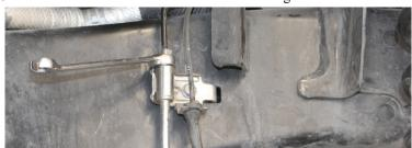
4. 10mm - Remove the factory brake line bracket from the frame.
