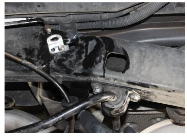
4. Insert the carli brake line through the guides and tighten them to the hard line through the new installed frame bracket.
