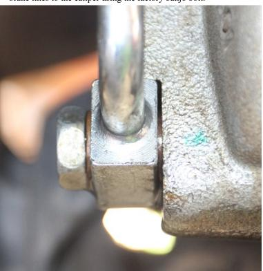
Ensuring all is installed and routed properly, tighten the factory hardline to the Carli line and install the clip to secure the brake line to the frame bracket.
