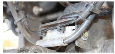
2. Separate the factory brake line from the ABS line as the brake lines will be replaced.
