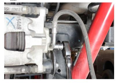
3. 16mm - Remove the two bolts securing the sway bar mount to the frame and slide the provided brake line guides into place resecuring them with the factory hardware. The guides index forward of the mount and the routing hole/grommet will shoot from the inside out at a 45° downward angle routing the brake line inward of the sway bar. They ARE side specific. Use the factory hardware to secure the provided brake line bracket to the frame.
