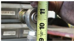
6. With the upper and lower heim joints clocked parallel to each other, tighten the jam nuts to affix the end link's configuration.
