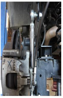
From the outside - in, The upper will be arranged: Sway Bar Link, Washer, Sway Bar, Flange Nut. Torque to 75lb.ft. NOTE: 17MM wrench holds rod end from spinning while you torque the nut.
