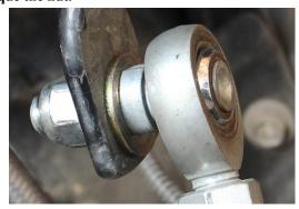
10. From the outside - in, The lower will be arranged: Sway Bar Link, 1/2" Gold Spacer, Axle Mount, Washer, Nyloc. **Torque to 75lb.ft.**
