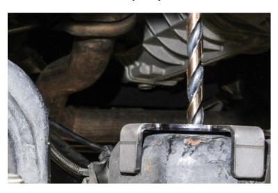
Once drilled, install the bump riser provided with your shock package; the short meant for the 2.0" IFP and Remote Reservoir will measure 5/8" and the tall meant for the 2.5" Remote Reservoir will measure 1-3/8". The Bolt is a 3/8" and the socket used will be a 9/16". Place the bump riser on the drilled surface, insert the bolt into the recess on the bump riser and slide the washer and crimp-lock nut to the underside of the lower spring bucket. Torque to - 20 lb.ft.
