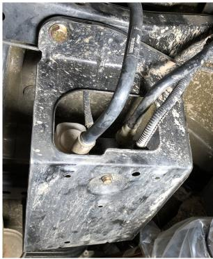
Up Front, drill the 2nd 1/2" hole all the way through the crossmember and use the 2nd 1/2" bolt to secure the 2nd mounting location.
