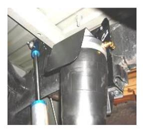
**20.** Pry back brake line loop on passenger side and tap flat against the axle.
