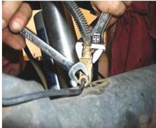
**8.** Retighten brake lines. Install supplied vent tube relocation fitting pointing it towards the front of the truck. Tighten fitting at both points.
