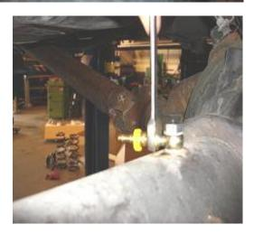
**9.** Mount upper air bag brackets to inner frame rails using supplied bump stop bolts. Be sure to route the wire harness over the top of the mount on the driver side.
