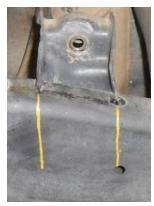
**10.** Cut the stock passenger shock mount off of the frame and clean for the new shock mount.
