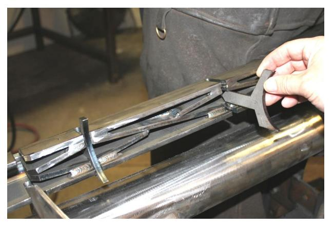
5) Attach the 2"x6" plates to the ends of the Axle Truss and apply a small stitch weld about ¼" long. Use these plates to help secure the truss to the axle with a C-clamp or other clamping method.
