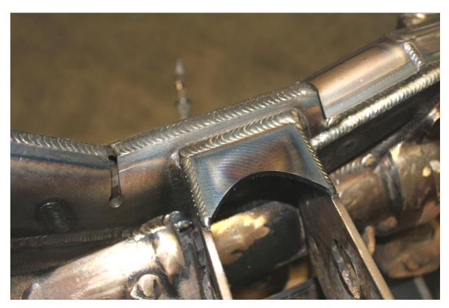
9) Install the Upper C Gussets, paying attention to how the plates fit between the C's and the coil buckets. For strongest install, wedge the gussets BETWEEN the Upper C Forging and the coil bucket. Try to avoid placing them on the outside of the Upper C Forging.
