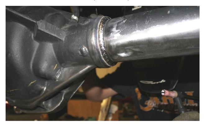
4) Remove Truss from Box and break off the 2"x6" plates from ends. SAVE FOR NEXT STEP. Slip the pre-welded Truss up to axle and check for fitment. Relieve and trim any areas that require attention. Once the fitment is
