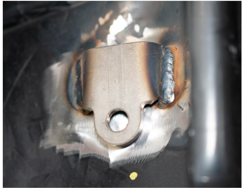
15. Use a jack to compress the axle upward 2"-3" and attach the limit strap to the upper tab until mostly tight - you still want it to be able to pivot by hand.
