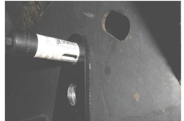
9. Insert the ½" x 4" Bolts with washers and nuts. Leave the bolts loose.
