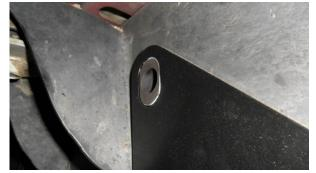
Some trucks might need some slight grinding on the oval frame hole, the radius drop oval hole, or both to allow the oval crush sleeve to go all the way through. BE CAREFUL WHEN GRINDING. Use a rotary file or stone, and only grind a little at a time. The oval crush sleeve needs to have a tight fit in the oval hole. It is preferable to have to tap the Oval Crush Sleeve into the frame.
