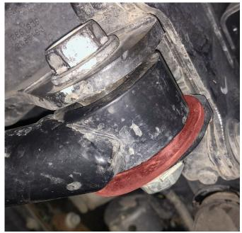
NOTE: Factory height trucks will require the track bar to be set to 38-7/8". This measurement is also applicable to any lift that utilizes a track bar drop bracket meant for the factory track bar.
