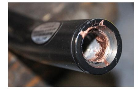
11. Thread the provided jam nut all the way to the end of the shank on the heim-joint so it's tight against the housing. Thread the heim joint 1-2 threads into the track bar. Apply RED LOCTITE to ALL the exposed threads of the track bar. These are the threads on which the Tapered-Jam Nut will sit.
