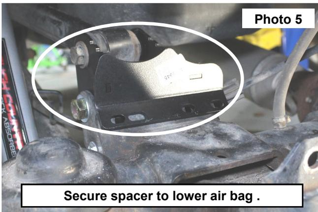
Secure spacer to lower air bag .
