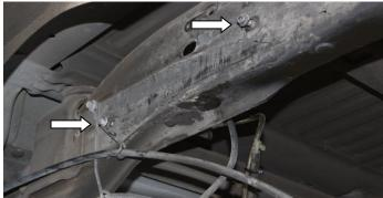
6. Fit the passenger side bracket up to the frame rail and use the provided 3/8" x 1" hardware to hold it in place to the bottom of the frame rail, hand tight.
