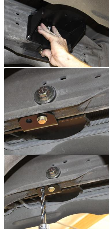
**NOTE:** When Drilling on the DRIVER'S side, there are fuel lines running the length of the frame rail. Remove the fastening hardware and move these lines out of the way if not already moved from installation of the 5/8" hardware.
