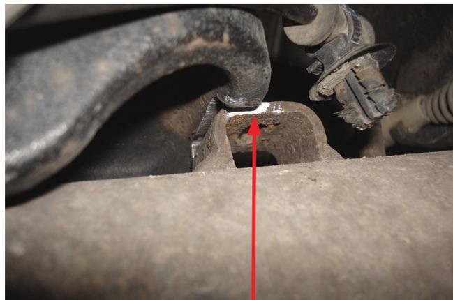
Grind strike plate so that there is clearance between the ABS bracket and strike plate when spacer is sitting on the spring perch.
