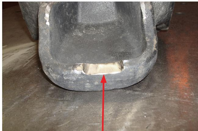
Grind out area between marks made from ABS bracket as shown.
