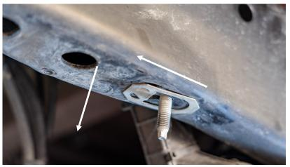
6. Install the captured-nut bracket in the frame. The threads face up and doublers that fit the cutout face down and index the bracket into the openings.
