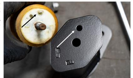
5. Remove the factory studs from the holes in the frame rail. Pull down and inward (toward the center hole) to remove them.
