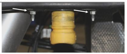
3. Remove the bump stop from the factory plate and retain the nut.
