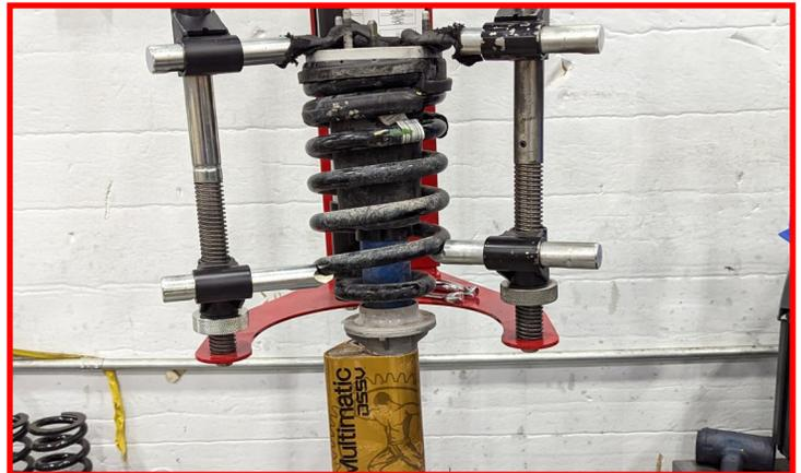
When there is enough room, install the two halves of the preload spacer, combining them together around the shock body. Plastic spring seat should be above the preload spacer.
