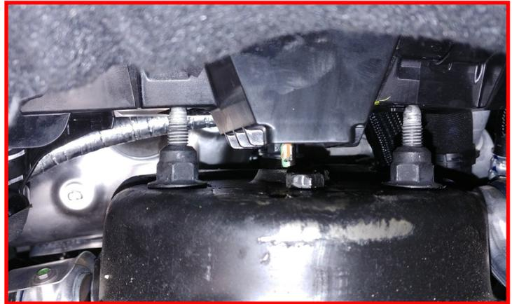
Support the **knuckle** with a jack stand. Remove **strut to lower control arm bolts**.
