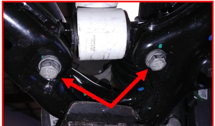
Install the factory nut on the sway bar end link. Torque **sway bar end link lower nut** to **45 ft-lbs**.
