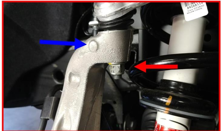
Loosen but do not remove the lower control arm pivot bolts.
