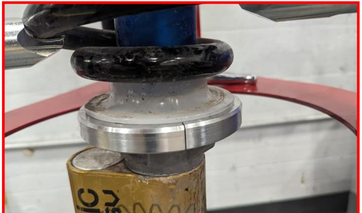
Relieve the spring pressure and remove from spring compressor.
