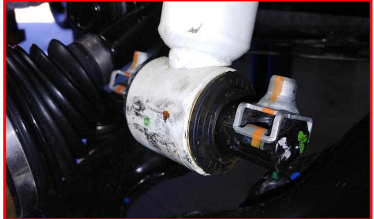
Remove **factory upper control arm** from vehicle and **discard factory arm**.
