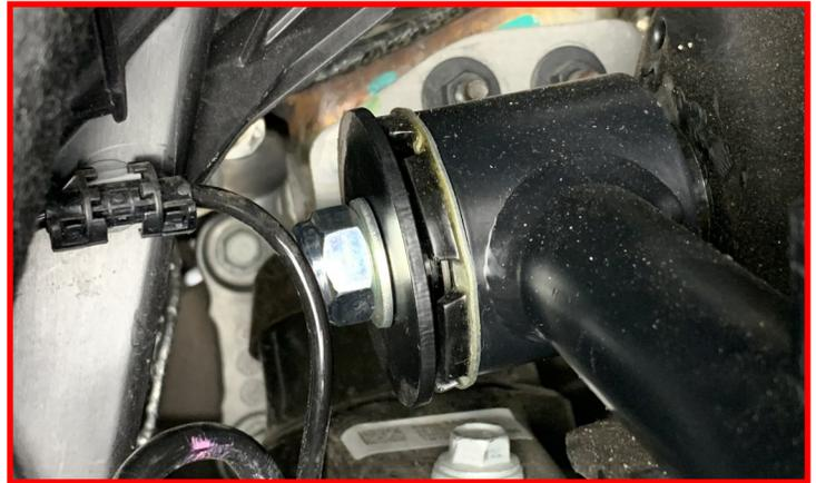
Using a spring compressor, compress the bottom of the spring until there is enough room under the spring to install the preload spacer. Ensure that the shock body does not rotate in relation to the top mount during this process.
