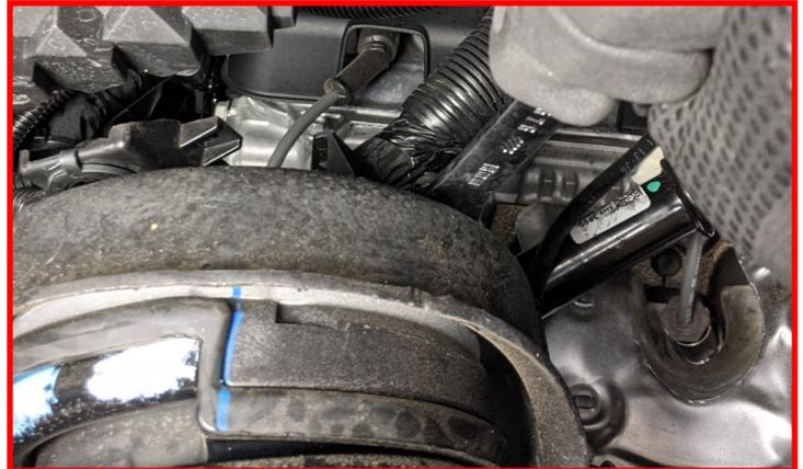
Torque **strut to lower control arm bolts** to **45 ft-lbs.**
