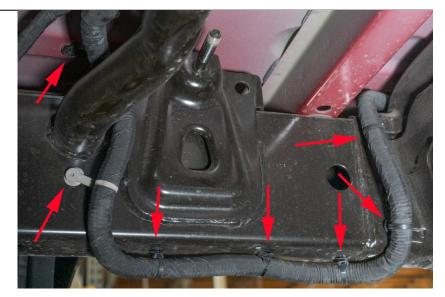
3. Remove the factory rear "stud" from the OEM Shock mount. We use a cutoff wheel to remove the stud, then a flap disk on a grinder to level the remainder of the stud to the factory bracket. Clean all areas to be welded. Mocking up the shock mount to the existing two holes In the factory bracket will allow you to trace the weldpaths.
