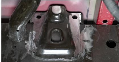
4. Insert the 2.75" width crush sleeves into the factory driver's side shock mount and the 3.0" into the passenger's side mount. Retain the crush sleeves into the factory holes by inserting the provided 1/2"x4.5" hardware with a washer on the bolt head from the outside set of holes to the inside. NOTE: If you have a factory or aftermarket 5th wheel hitch that uses these holes, you can reuse the hardware already installed OR replace it with our hardware.
