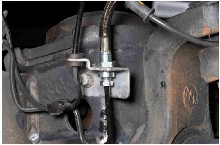
12. Slide the factory hard line into the Carli bracket and secure it to the radius arm bracket with the factory hardware. Once in position, use the factory clip from the discarded bracket to fix it's position.
