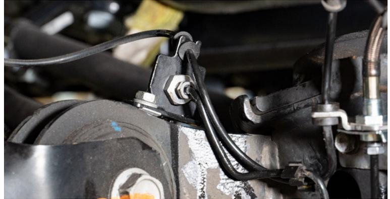
*Brake Line Routing on Caliper*
