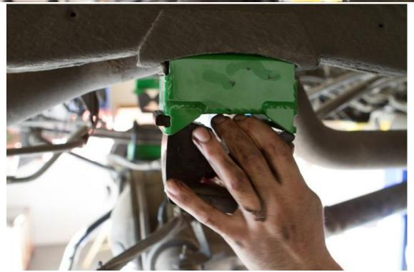
26) Once the second side is started, a screw driver, some wiggling and some additional lubricant will be needed to get the bump stop fully seated in the bracket.
