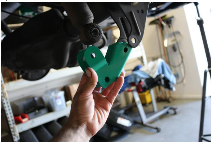
29) Install M8-1.25 x 65mm long bolt provided as shown above to locate bracket in place. Use a washer under the bolt head.
