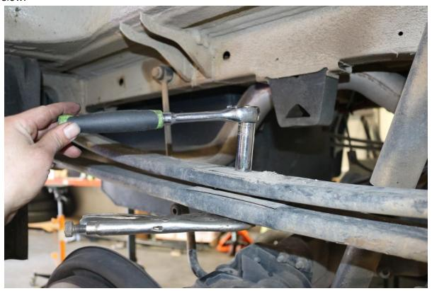
14) Next disassemble the add-a-leaf pack by using a 9/16" socket / wrench to remove the leaf spring center pin nut and a 5/8" socket / wrench for the spring clamps. Retain all hardware.
