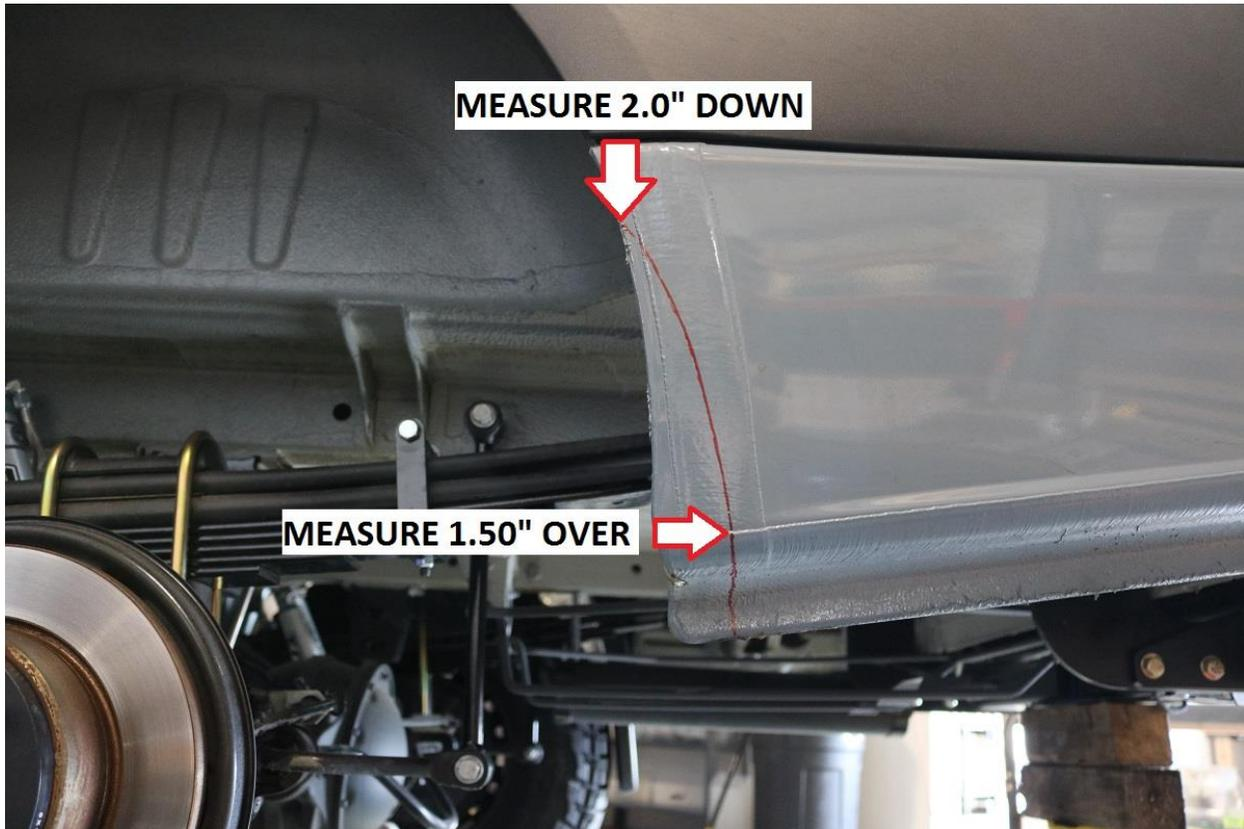
45) Using the line marked above as a guide, cut the fender using a 4-1/2" angle grinder with cut off wheel.
