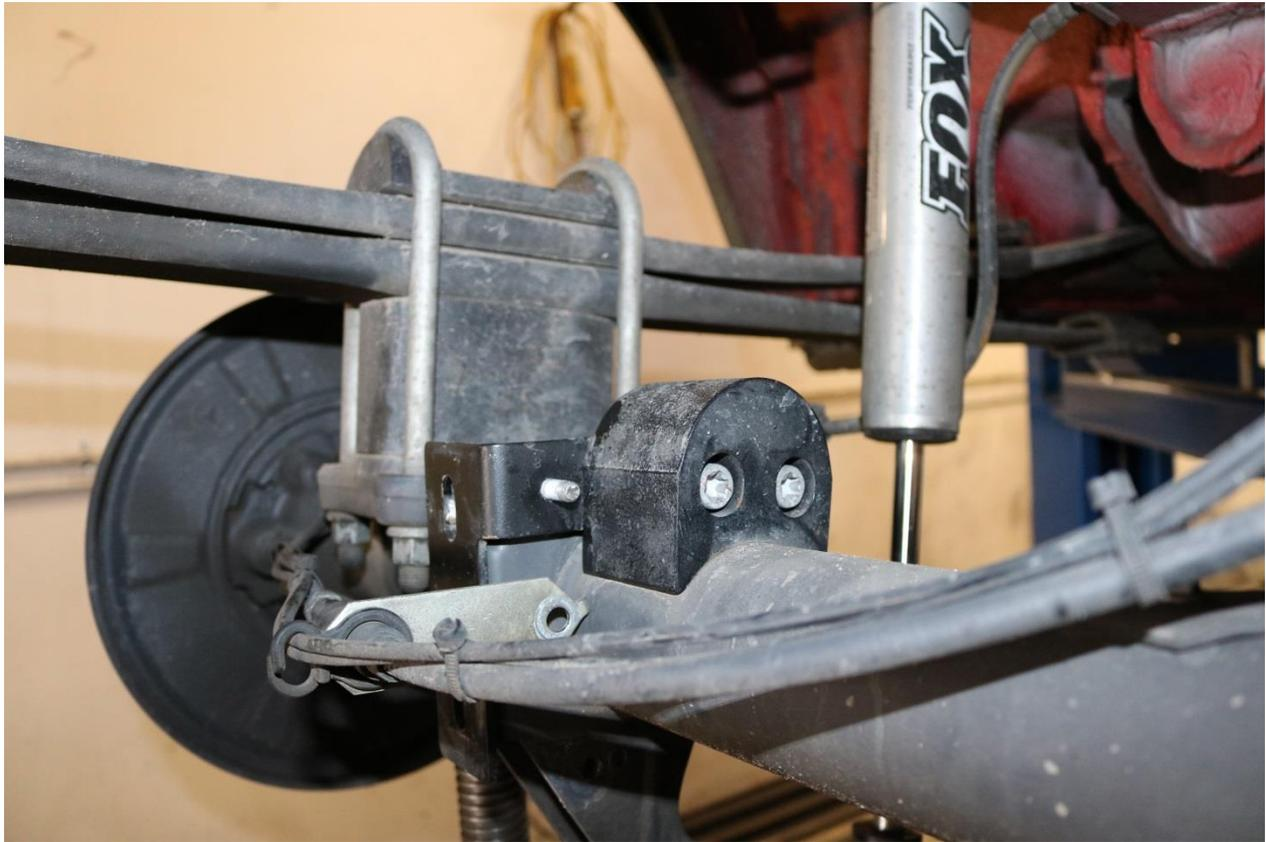
35) Re-install the rear sway bar onto the axle. Use the four T55 Torx bolts removed in step 6. Torque to 52 ft-lbs (70 N.m).
