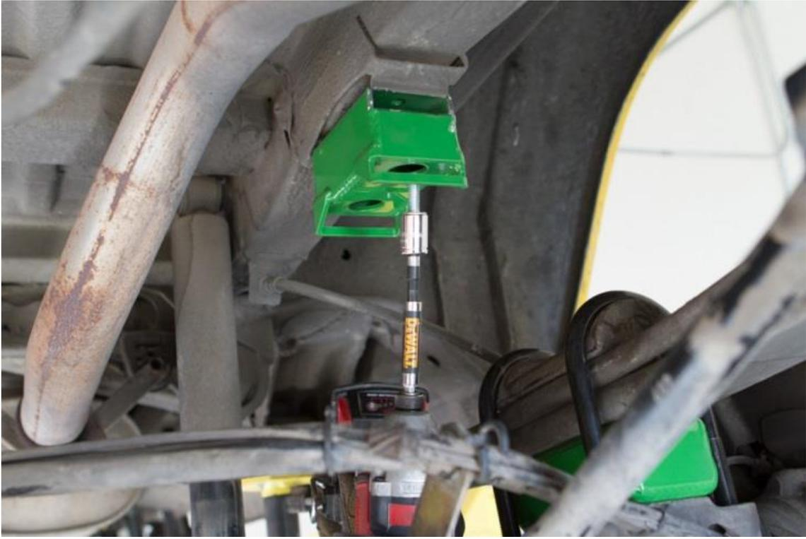
23) Use drill / driver to snug bolts into place. Do not fully tighten using drill / driver. Torque bolts to 13 ft-lbs (17 N.m).
