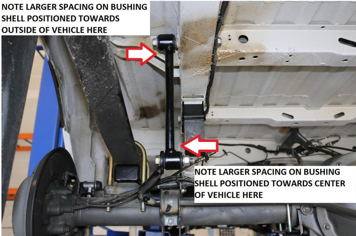
**NOTE LARGER SPACING ON BUSHING SHELL POSITIONED TOWARDS CENTER OF VEHICLE HERE**
