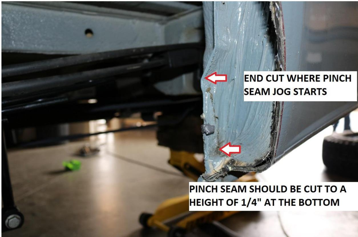
46) Sand smooth any rough cut edges and paint any exposed areas of metal to prevent corrosion. Below is an example of the finished cut fender prior to painting.
