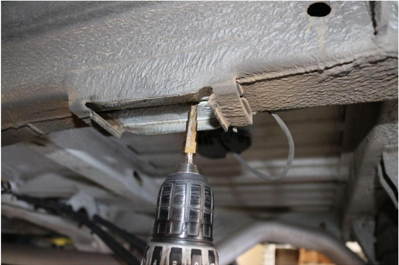
22) With both holes drilled, position the bump stop drop bracket in place and secure it to the chassis using the 5/16-18 x 1" long thread cutting screws included with the kit. Use a nut driver or drill with a 1/4" bit adapter and a 1/2" socket to install the screw. Try to keep the drill / driver as straight as possible when cutting the threads.
