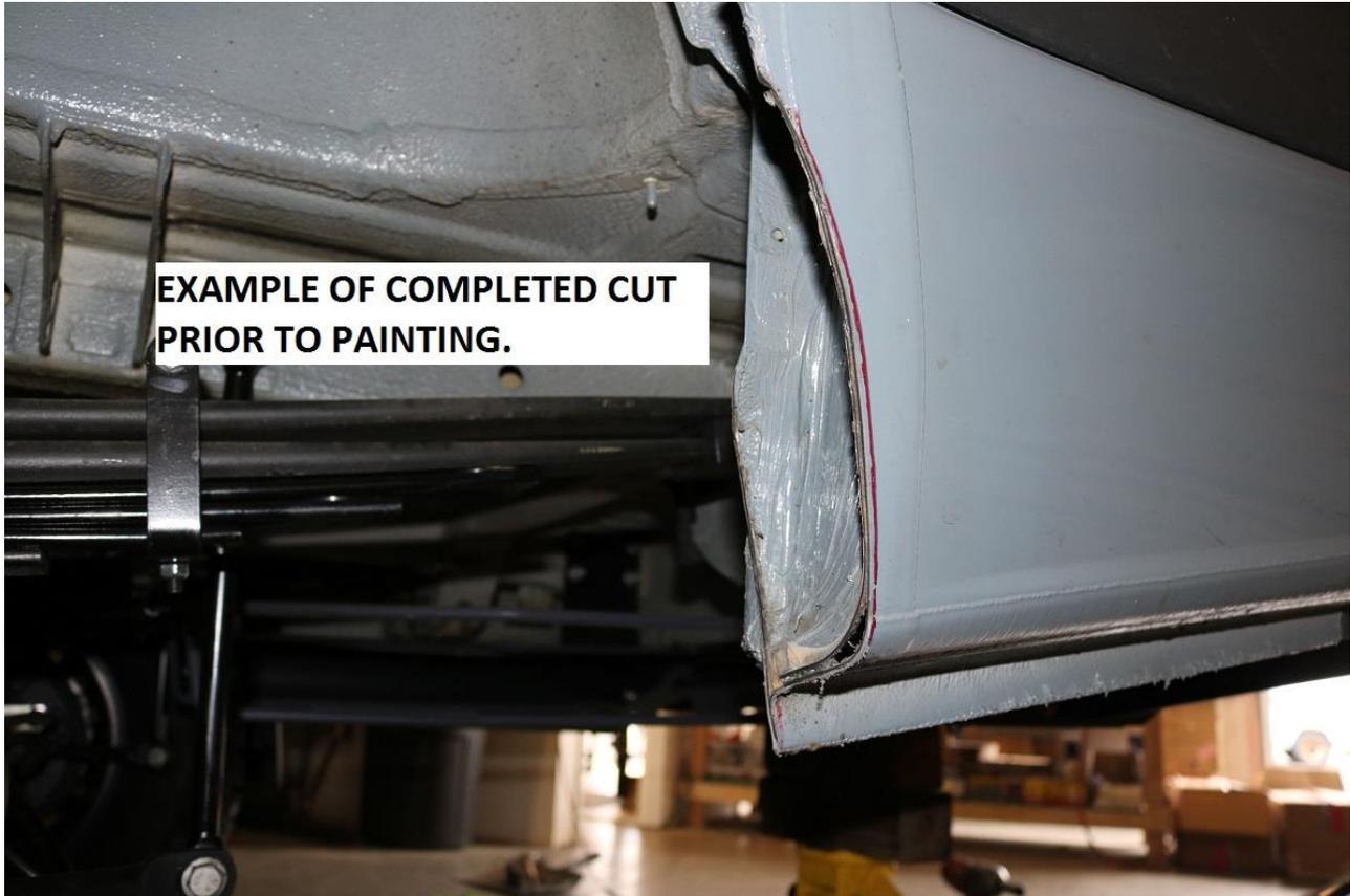
47) Trim the rear mudflap as shown in the image below. A pair of tin snips or quality scissors works well for trimming the mudflap.
